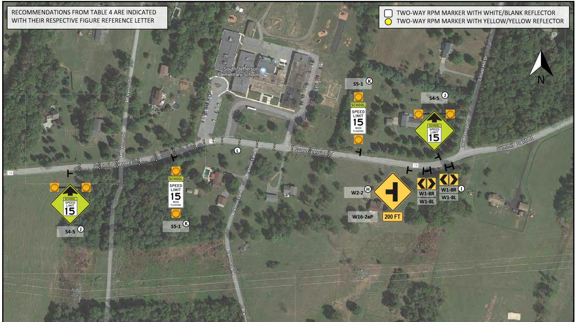
Figure 6: Signing and Pavement Marking Recommendations for Locust Hill Drive Intersection and School Zone Area
