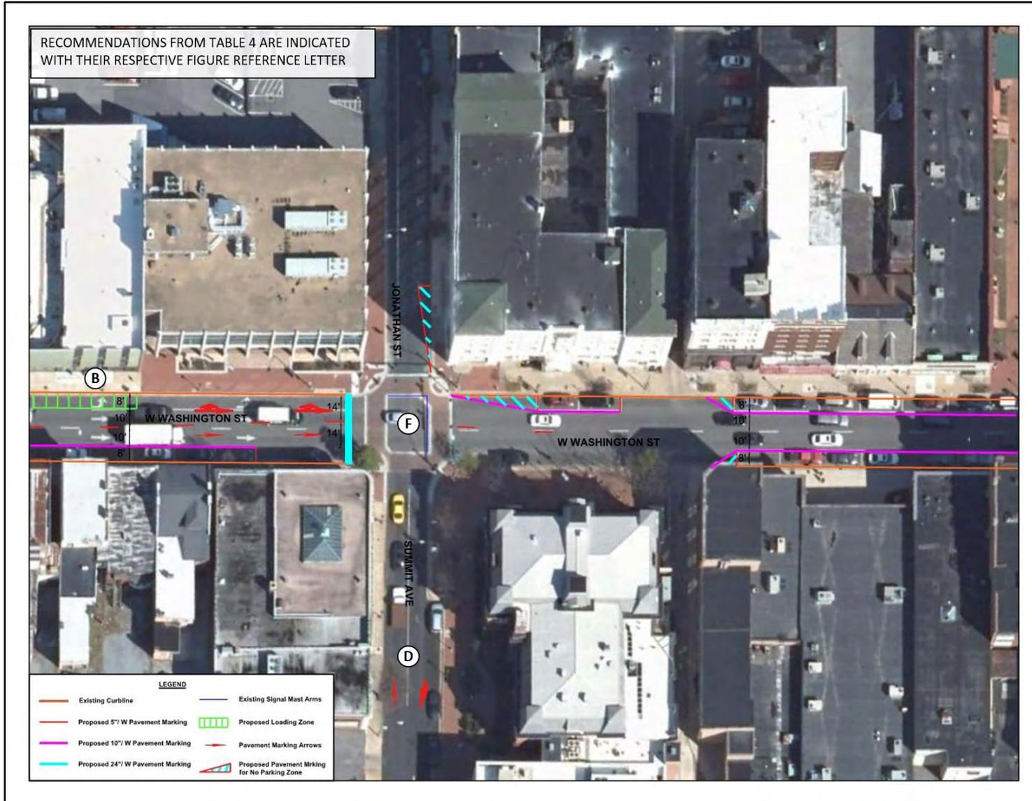
Figure 8: Pavement Marking Recommendations at Washington St/Potomac St Intersection
