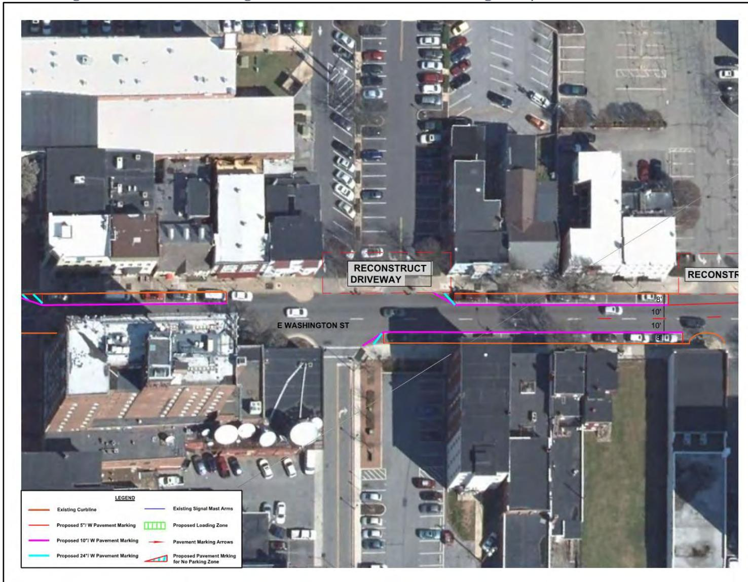
Figure 10: Pavement Marking Recommendations at Washington St/Locust St Intersection
